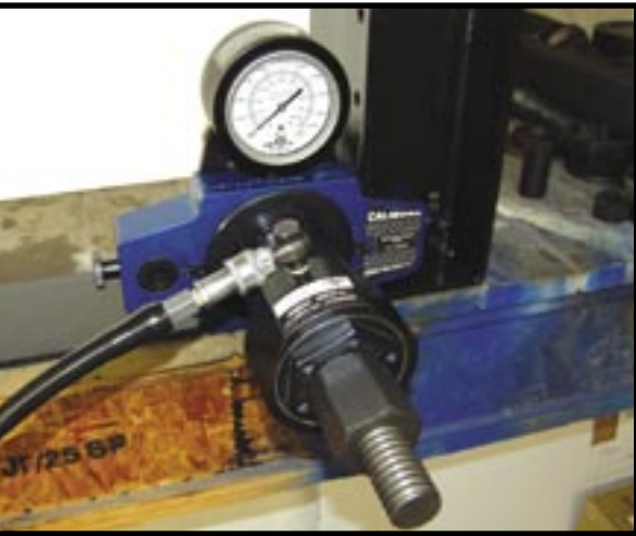
Use with T-Con base bolt tensioner.
